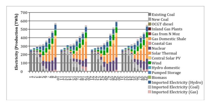
Figure 4 Electricity production in TWhs for 10 and 12 Gt constraints, compared with CTL output fixed to 2040 (SAS scenarios)
