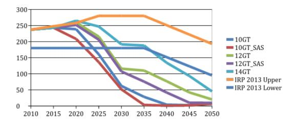
Figure 8 Comparison of carbon constraints in the Integrated Resource Plan update and those applied in the current study
