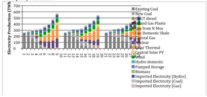
Figure 3 Electricity production under 14, 12 and 10Gt CO<sub>2</sub>-eq constraints
