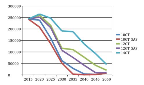
Figure 2 Carbon constraints applied to the electricity sector in each scenario
