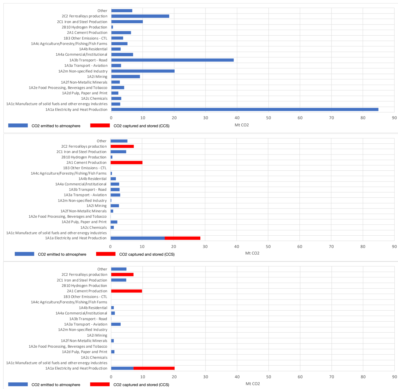
Figure 27 – Remaining CO 2 emissions in 2050 in the reference case (top), net zero 45 Mt sink case (middle), and net zero 20 Mt sink case (bottom), and use of CCS. The overall length of the bars in each category are the CO 2 produced by that sector in 2050; the red section of each bar is the amount of CO 2 which is stored, and the blue section is the amount emitted to atmosphere.
